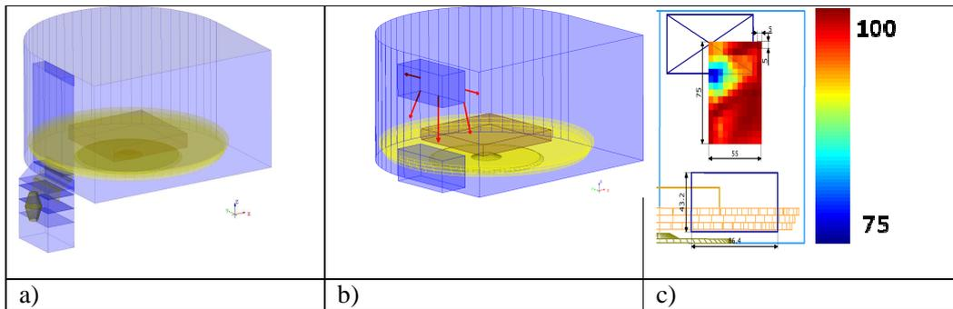
Figure 1. The Whirlpool MAX oven: its original model (a), the model under optimization (b), and the highest-efficiency map for the top waveguide scanned across the side cavity wall (each square marks one of the considered 165 positions of the aperture center).
